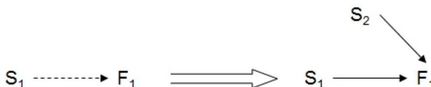
Fig. 2. Su-Field model describing X-ray phase-contrast imaging technique. Conventional X-ray attenuation leads to poor image quality when the sample S_1 is weakly absorbing. In order to enhance image contrast, local phase distortions of the X-ray beam (field F_1 ) passed through the object S_1 are detected by the phase-sensitive component S_2 . Phase differences are then converted into corresponding changes in amplitude that can be distinguished
